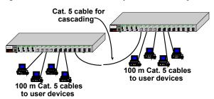
safety margin of 2 was used. Figure 3.6.1a: Two cascaded Magnum 8000X hubs
